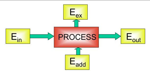
E<sub>in</sub>: Energy Content of incoming mass flow (products, gases, water, etc.)
